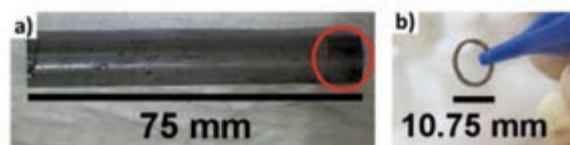
Fig. 1: Pictures of the irradiated plenum Zircaloy-4 cladding: (a) dimensions, the red circle indicates the welded end-plug; (b) a subsample prepared for a dissolution experiment.
