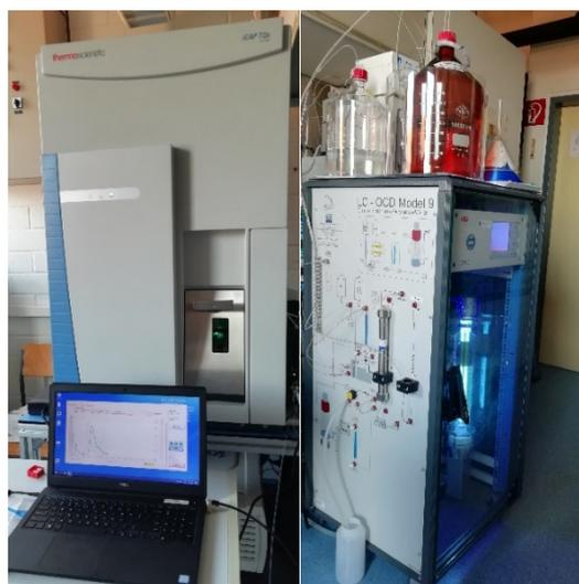
Fig.2: The hyphenated LC-OCD-UVD-OND equipment based on the liquid chromatography principle coupled to our new iCAP-ICPMS detector (KIT-INE, Status July 2021).
