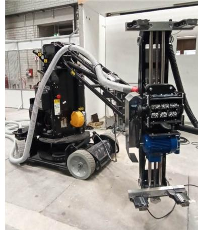
*Fig. 4: Manitou platform with shaver tool*
