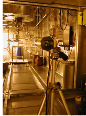
Fig. 4 Thermovision camera in the hot cell V3 viewing into melter cell V2
