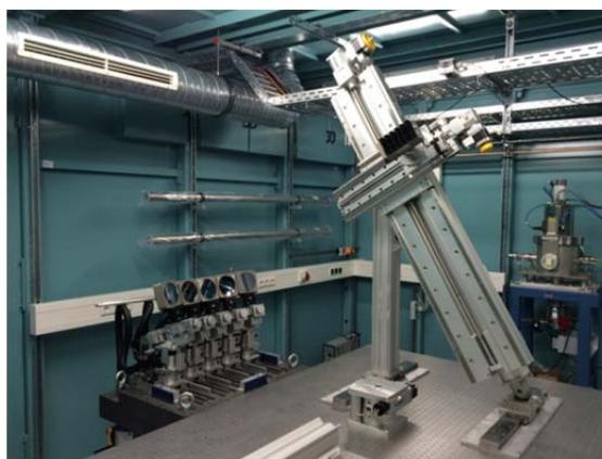
**Fig. 2:** The multi analyzer crystal HRXES spectrometer was transferred from the INE-Beamline and is now installed inside the ACT experimental hutch (Exp1).
