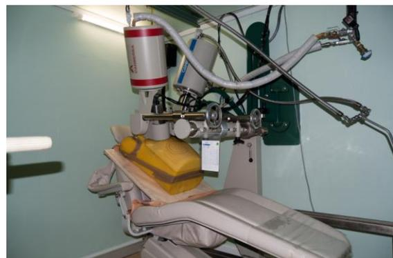
*Fig. 7: Measurement setup of the Livermore phantom performed in CIEMAT.*
