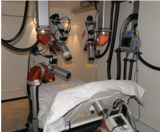
**Fig. 5:** The in-vivo counter at KSM-IVM in a whole body counting geometry
